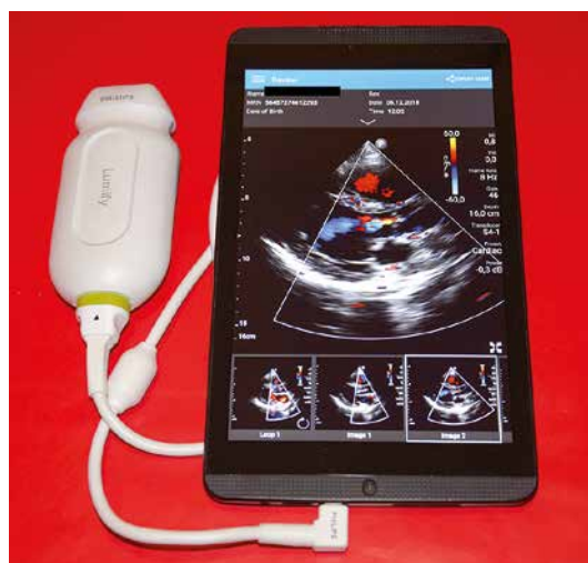
Figure 1. Personal mobile device-based pocket echocardiograph – microUSB probe S4-1 connected to a tablet
