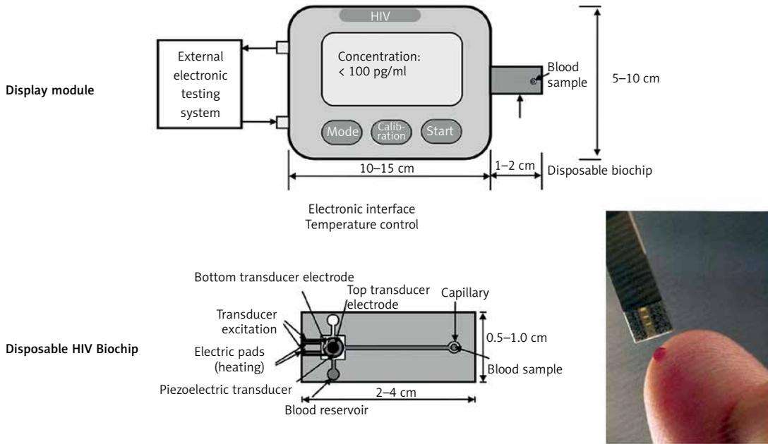
Figure 1. Display module of HIV Biochip cross-section (top view)
