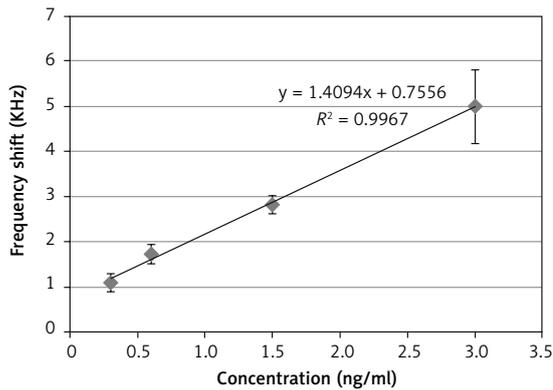
Figure 4. p24 detection sensitivity curve
