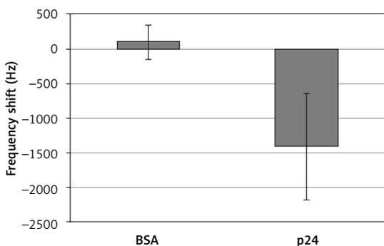
Figure 2. Antigen specificity. Binding of p24 versus BSA to sensor-anti-p24 interface. In this system a positive signal generates negative inflection
