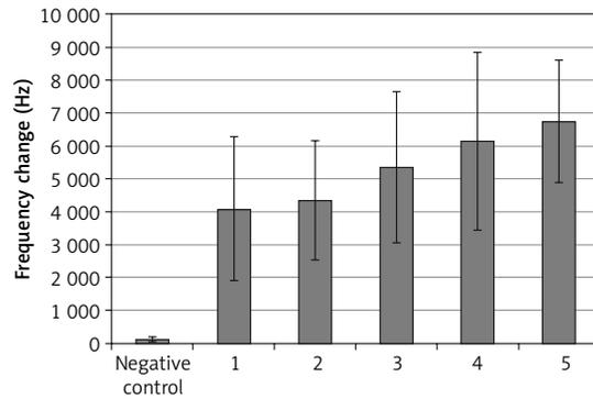
Figure 5. Bionanosensor analysis of HIV detection in human plasma samples (1–5)
