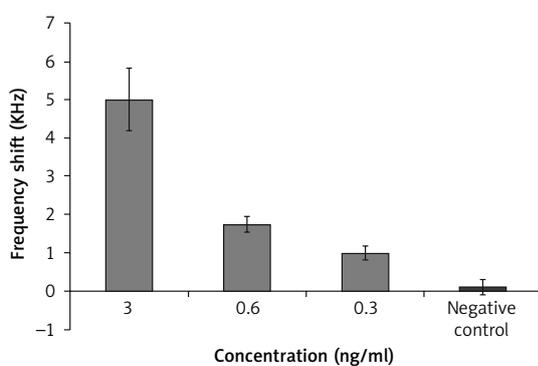
Figure 3. Frequency shift as a function of p24 concentration. Negative control – 5% BSA
