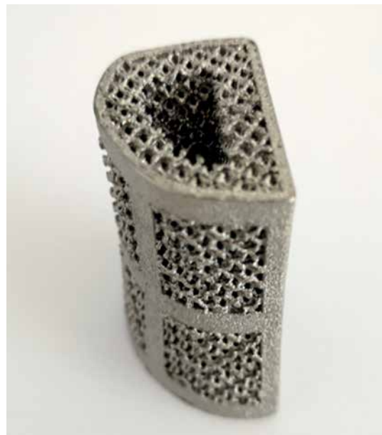
Figure 4. The final product of the 3D printing assisted artificial vertebral body
