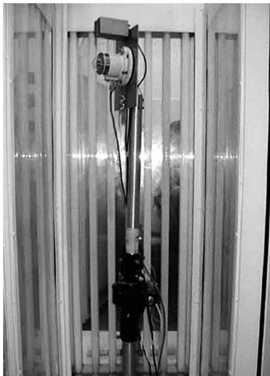
**Figure 3.** The calibration meters mounted on a vertical plate that is attached to a rotating vertical beam. Its rotation is due to the motorized system (bottom)
