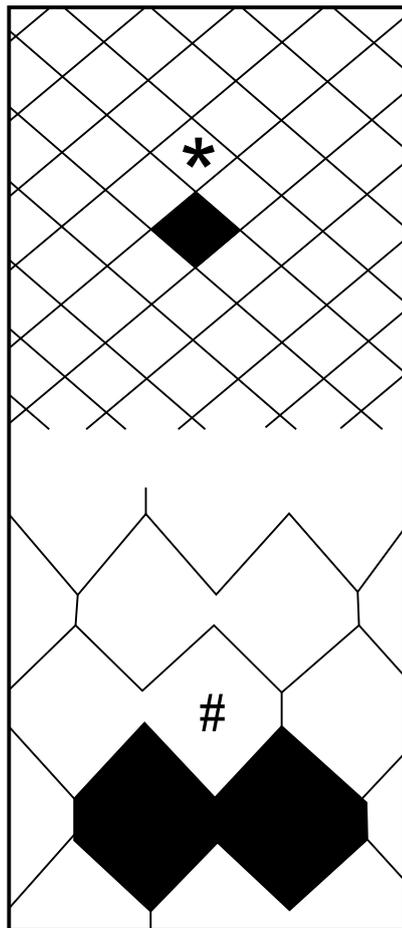
**Figure 1.** Schematic view of stent-cell designs: (\*) – closed-cell design vs. (#) – open-cell design
