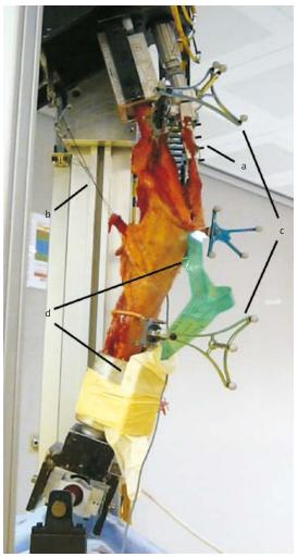
**Figure 1.** The experimental set-up with a cadaver specimen mounted on the knee rig, ready for a squat. The rig allows  $6^{\circ}$  of freedom for the knee joint. Visible are the clamp fixed to the quadriceps tendon (a) and cables attached to medial and lateral hamstring tendons (b); the marker frames on tibia and femur (c) and the Tekscan sensor and handle (d)
