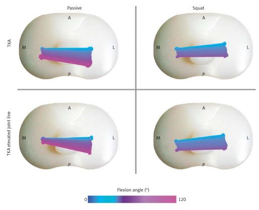
**Figure 2.** Top view of the tibial insert with the medial and lateral femoral condyle centers projected onto it during the different motion cycles (passive cycles on the left, squats on the right). Top row shows knee kinematics after primary TKA with joint line reconstruction, lower row shows knee kinematics after revision TKA with 4 mm joint line elevation
