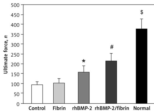
**Figure 7.** Ultimate force of the lengthened segments and the contralateral tibiae in the control group 8 weeks after drug treatment were measured by three-point bending test
