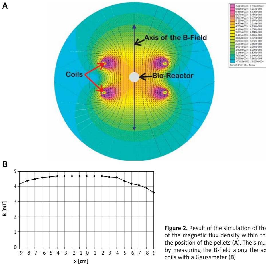
**Figure 2.** Result of the simulation of the spatial distribution of the magnetic flux density within the Helmholtz coils in the position of the pellets (A). The simulation was validated by measuring the B-field along the axis of the Helmholtz coils with a Gaussmeter (B)
