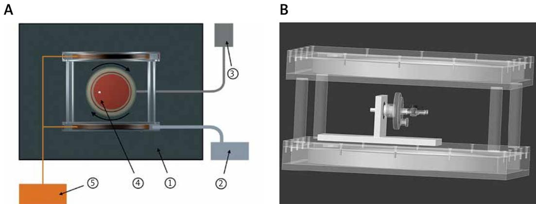
**Figure 1.** SMG/LF-EMF bioreactor system: **A** – Schematic drawing of setup compounds: incubator (1), LF-EMF solenoid with external cooling system (2), external motor gear of the SMG (3) connected to RCCS vessel by a flexible shaft, floating pellet (white) within the RCCS vessel (4), external frequency generator of the LF-EMF (5). **B** – Drawing of the position of the SMG bioreactor and RCCS vessel within the Helmholtz coils
